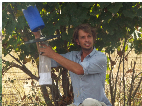
Photo on the left shows local field technician Skumbuzo Mdletshe setting up a light and CO 2 baited mosquito trap in Kruger National Park, South Africa
